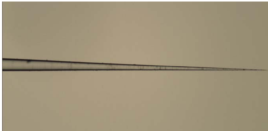
Taper coated with ITO, tip diameter 2 μm
