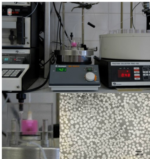
Fig. 5 System for preparation of liposomes by removal of detergent using ultrafiltration. A) photo of the system linked with FPLC; B) photo of the ultrafiltration cell in detail (pink: LR-PE-labeled liposomes inside the cell). (C) monodisperse liposomes prepared by detergent removal method. ( Analytical Biochemistry 408 (2011) 95–104).
