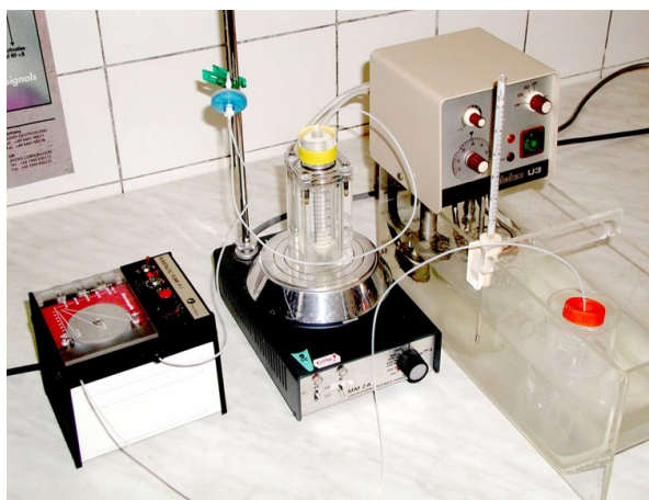
Fig. 7 Photograph of whole system with stirred and thermostated cell for sterile production of liposomes by proliposome-liposome method. (Methods in Enzymology 2003, 367, 110-125).
