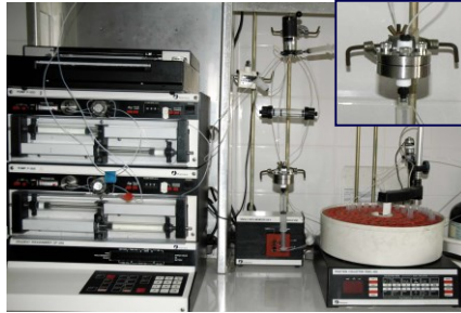
Fig. 9 Device for extruding liposomes by application of preparative FPLC system and using a high pressure extrusion cell. The system can be automated with the use of automatic metering valves and using two 50 ml "Superloop". Insert - detail of high-pressure extrusion cell (designed by author and made in workshops at VRI). (Analytical Biochemistry. 1994, 218, 352-357).
