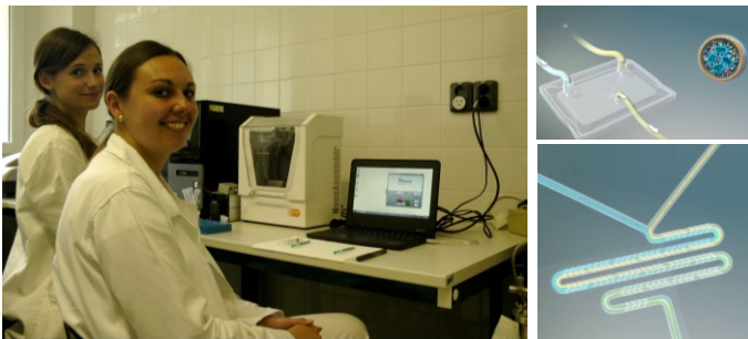
Fig.10 The instrument NanoAssemblr® in our laboratory NanoPharm. NanoAssemblr® (left), nanofluidic mixing chamber (middle); scheme of nanofluidic mixing (right).
