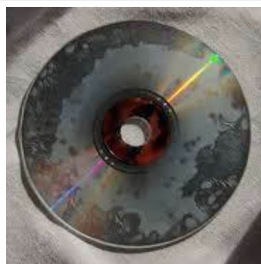
A CD after flooding.
