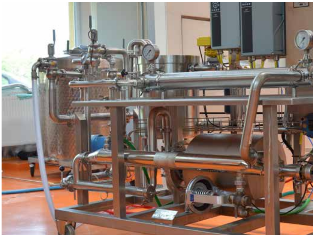
Cross-flow filtration: universal unit Alfa Laval M39/M3.8 for microfiltration, ultrafiltration,
