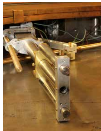
An adjustable beam outlet from the accelerator chamber
