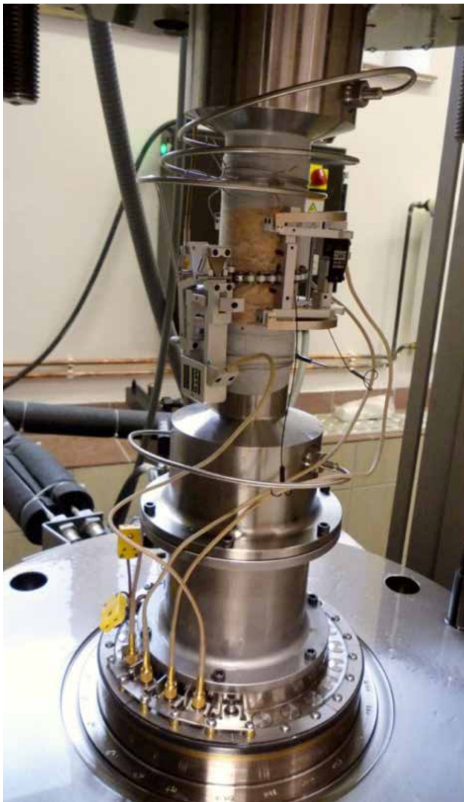
Setup for triaxial test of rock sample exposed to pore water pressure
