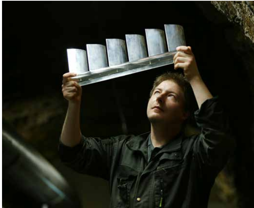
Technician Antonín Zajiček inspects the blade cascade model before mounting into the aerodynamic tunnel
