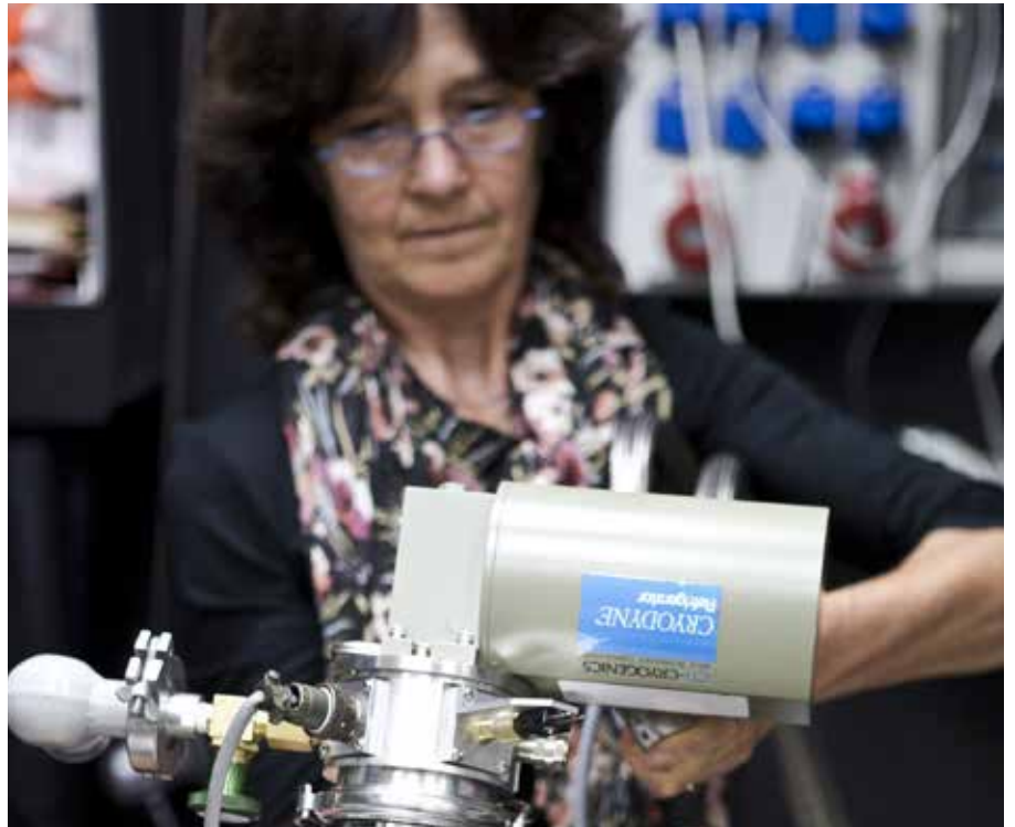
The cryostat head of a Janis closed-cycle refrigerator
