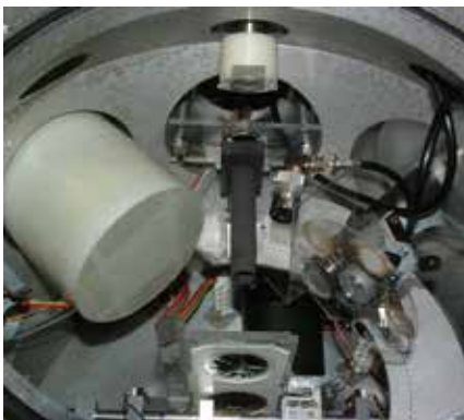
Multifunctional analytical vacuum chamber enabling to measure X-rays and recoiled ions concurrently
