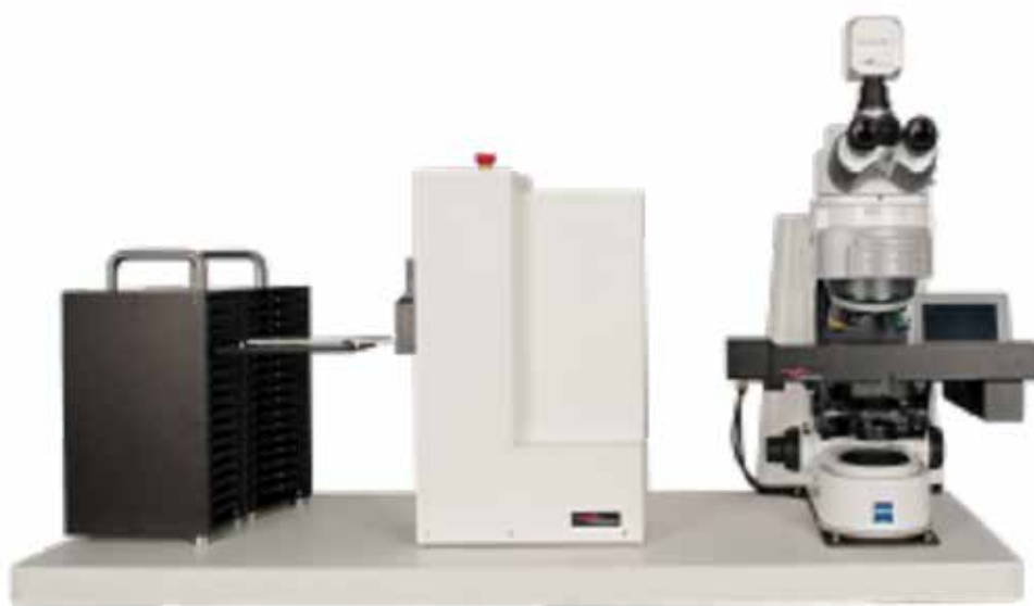
Metafer Slide Scanning System version 3.11., MetaSystems GmbH (Comet assay) for analysis of genotoxic potential of nanomaterials
