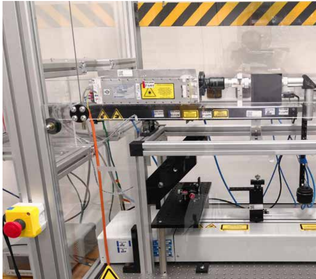
CO 2 laser for the preparation of special fiber components
