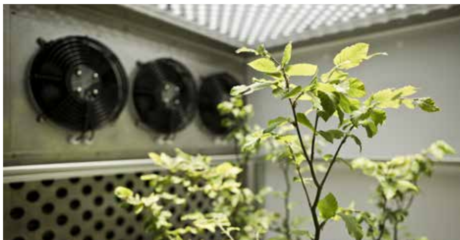
Growth chambers used for experiments assessing the global change impacts allow, in addition to regulating basic parameters such as air temperature or humidity, changing the concentration of carbon dioxide or the spectral composition of light
