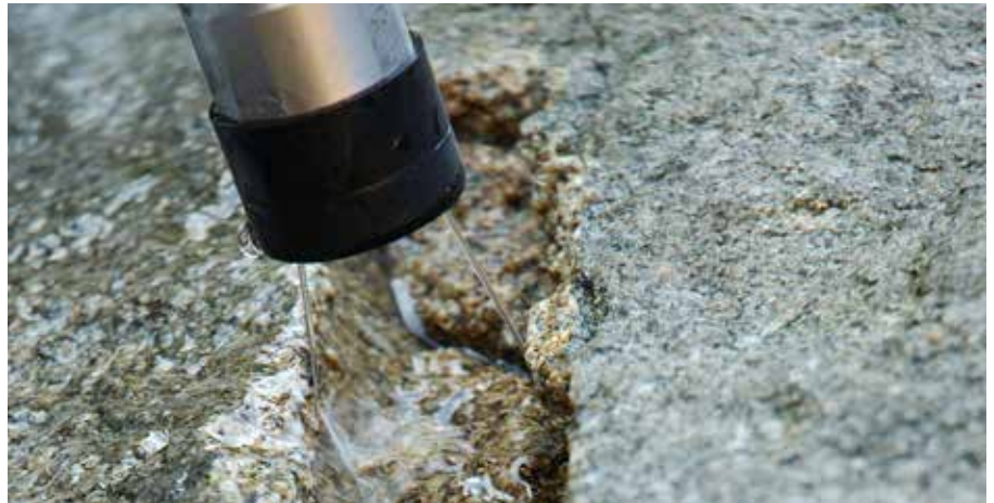
A kerf created by rotating pulsating high-speed water jet in granite massif (Erlich quarry, locality Žulová)
