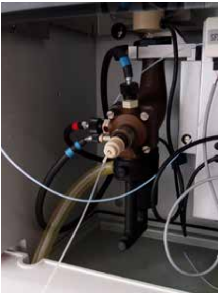
Detail of the nebulizer and the injection module SFS 6 of the Atomic Absorption Spectrometer ContrAA 700 (Jena Zeiss)
