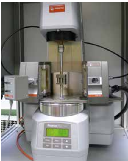
Rotational rheometer Anton Paar MCR 501 with an oven up to 400 °C and in-built camera
