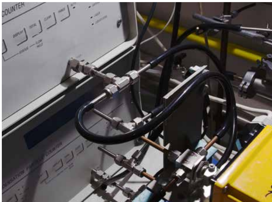
Aerosol particle counters – the brain of a set-up for measuring the efficiency of filters
