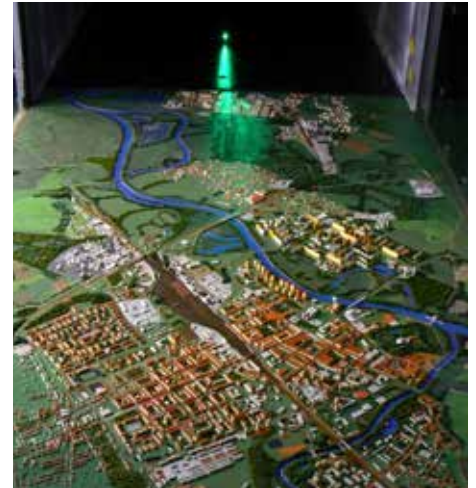
Visualization of the flow above the model of the city of Pardubice inside the wind tunnel
