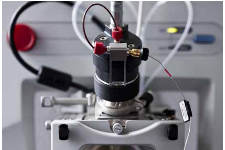
Metabolomic profiling as well as target analyses of organic molecules can be carried out thanks to the state-of-the-art gas and liquid chromatography equipment supplemented by high-resolution mass spectrometers (Orbitrap ionisation source)
