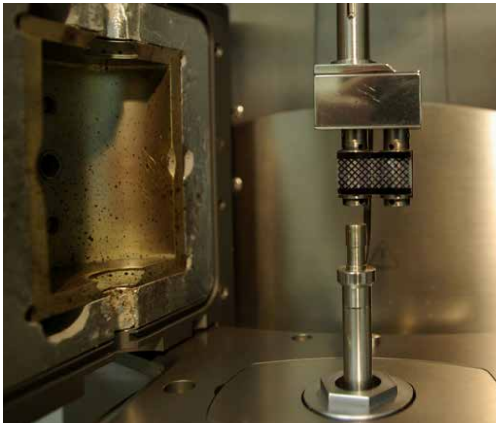
Sentmanat extension rheometer in-built in an Anton Paar rotational rheometer with an illustrative polymer sample
