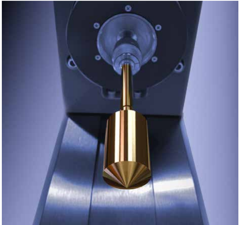
The concentric cylinder arrangement of the rotational rheometer
