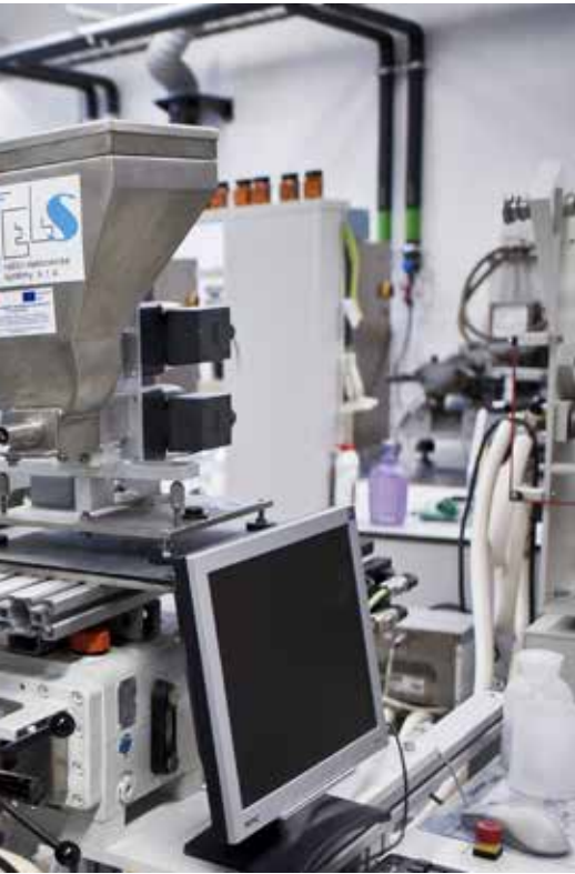
The Centre is equipped with a technology capable of processing high-abrasion materials and special materials at high temperatures (up to 450 ° C)
