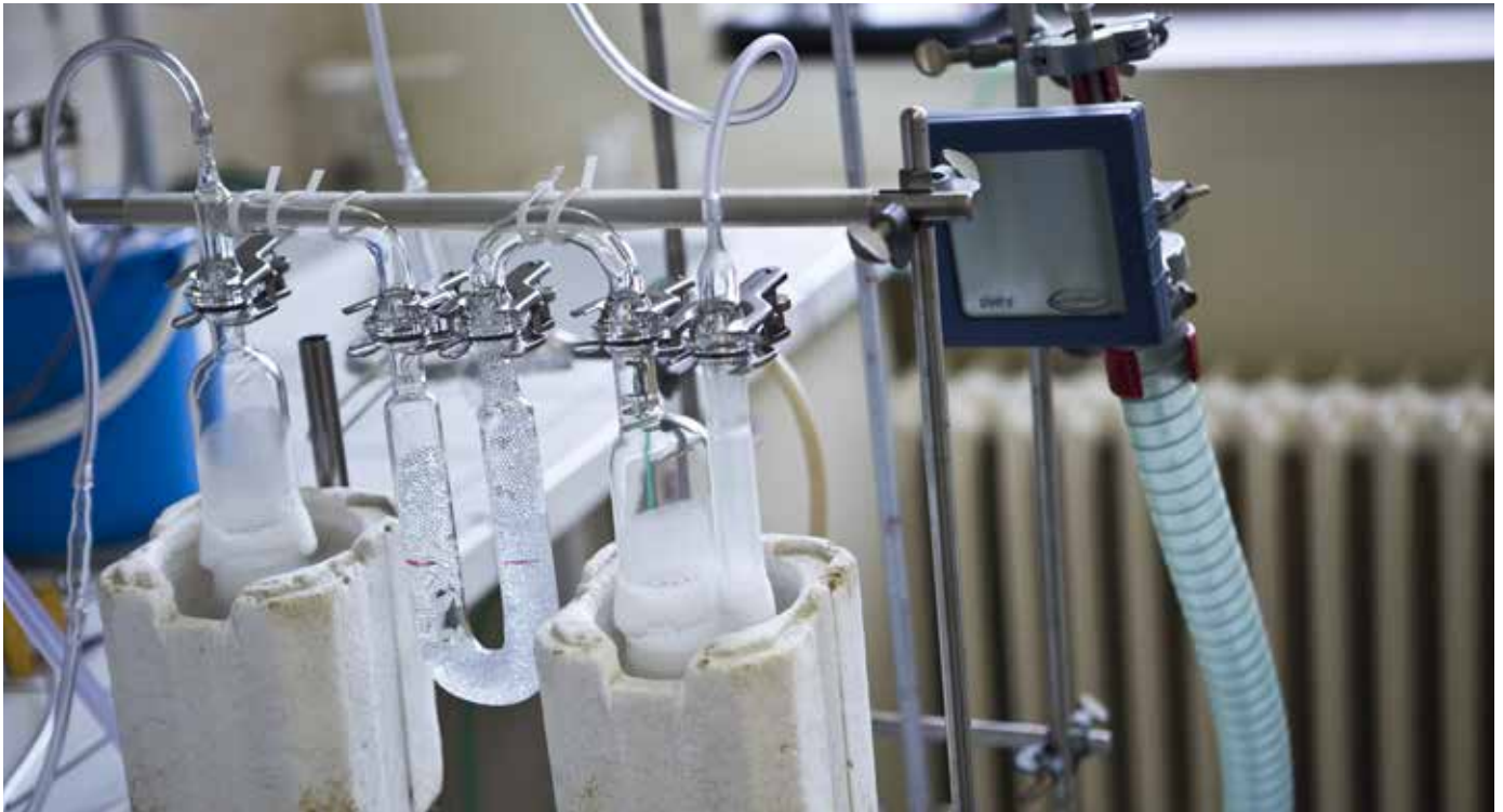
Transfer of C-14 to a chemical form suitable for the measurement of activity
