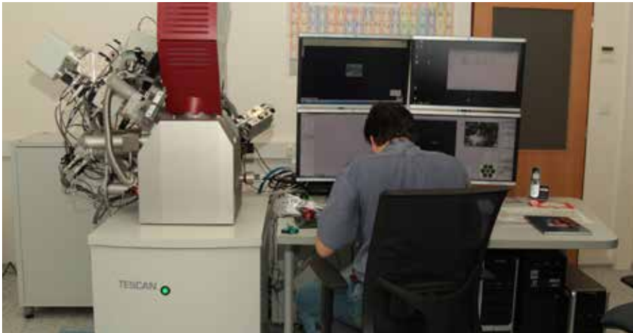
The TESCAN Fera3 scanning electron microscope with a focused ion beam for analysing the surfaces and microstructures of functional materials
