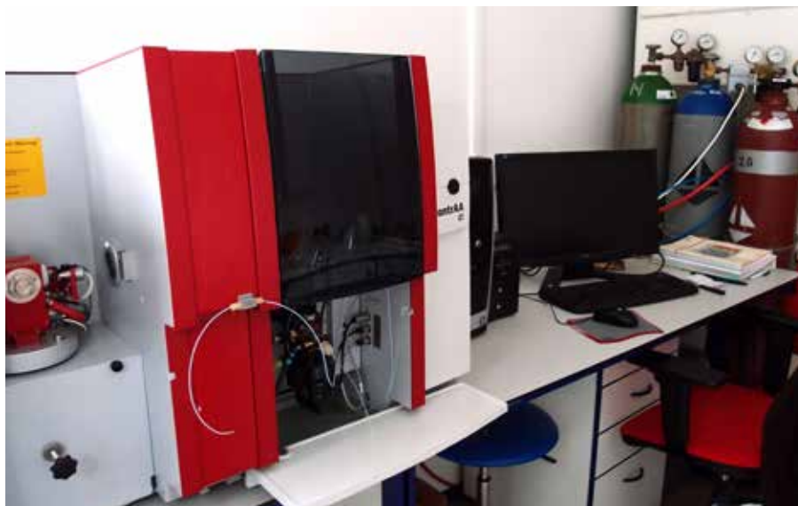
High-Resolution Continuum Source Atomic Absorption Spectrometer ContraAA 700 (Jena Zeiss) with possibility to change quickly from flame technology to graphite furnace technology
