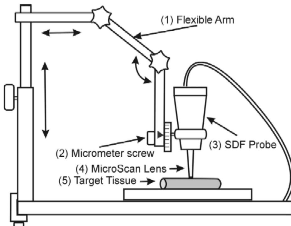
**Fig. 2.** A scheme of the stabilizing and fixation device for SDF imaging probe. (1) Flexible arm allowing horizontal, vertical and rotating movements ends with a special adapter with (2) micrometer screw for movement of the SDF probe (3) with MicroScan lens (4) within the range of 0.5 mm towards the target tissue (5).
