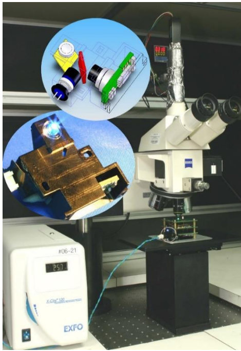
FIGURE 23 FLUORESCENT MICROSCOPE USED FOR OUR WORK WITH PCR SYSTEM UNDERNEATH IT.
