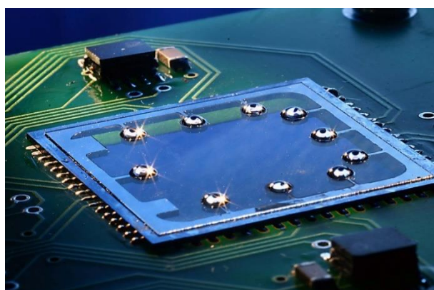
FIGURE 20 MINIATURIZED VERSION OF THE MICRO PCR SYSTEM, SO CALLED NANO PCR WITH VCRS WITH SAMPLE WITH VOLUME OF 100 nL.
