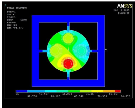
FIGURE 14 TEMPERATURE DISTRIBUTION AT THE SILICON CHIP AS MODELLED BY ANSYS. WE ASSUMED FOUR HEATERS WITH TEMPERATURE SET TO \approx 56 °C, TWO HEATERS AT \approx 72 °C A ONE AT \approx 93 °C.
