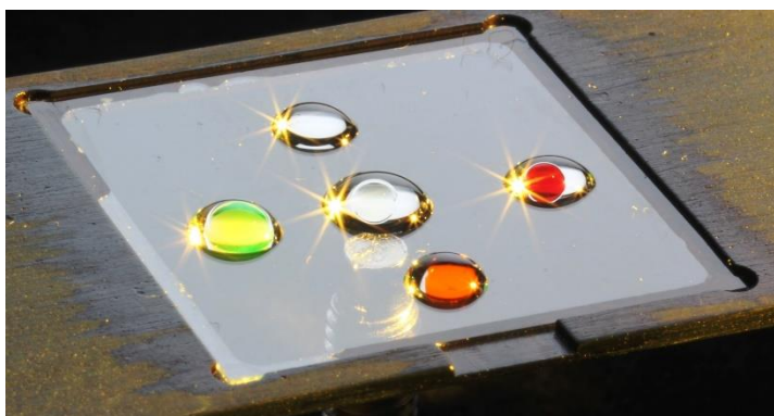
FIGURE 40 A PHOTOGRAPH OF A GLASS WITH 4 VRCs CONTAINING NUCLEOTIDES A, C, G, AND T (WE USED COLOR INK FOR CONTRAST ENHANCEMENT) SURROUNDING THE VRC SERVING AS WASHING STATION TO WASH DNA AND REMOVE DEBRIS FROM PREVIOUS REACTION.
