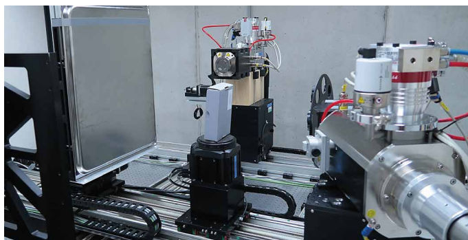
Figure 1: Accommodation of the box with the tablet in the TORATOM scanner.
