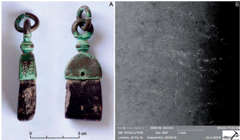
Fig. 2. A: Touchstone from the La Tène oppidum of Stradonice, Czech Republic (inv. No. KT00556 in the catalogue of the National Heritage Institute of the Czech Republic). – B: An example of streaks of an alloy of gold, silver and copper (tab. 1: 2). Microphoto: Š. Křížová. Courtesy of the NHI.
