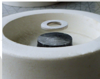
Model of a flywheel-superconducting bearing.
