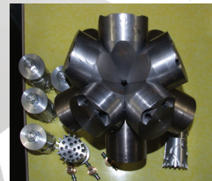
Magnetocumulative implosive plasma generator for direct conversion of plasma kinetic energy to electricity
