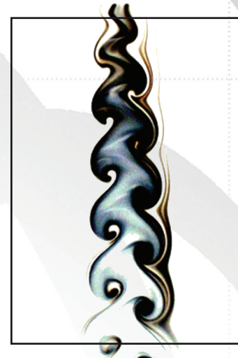
Wake flow behind a cooled circular cylinder (Von Kármán vortex street).
