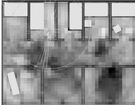
Fig. 1: Localization in simulation experiments. Room dimensions: 6x8m, 1600 samples, 72 beams, localization time 120ms, noise 20%
