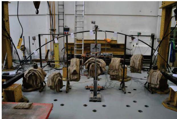
Fig. 1: Isolated arch under symmetrical loading (left); Comparison of experimental and numerical (SOFiSTiK) vertical deflections ( u_Y ) under symmetrical loading (right)
