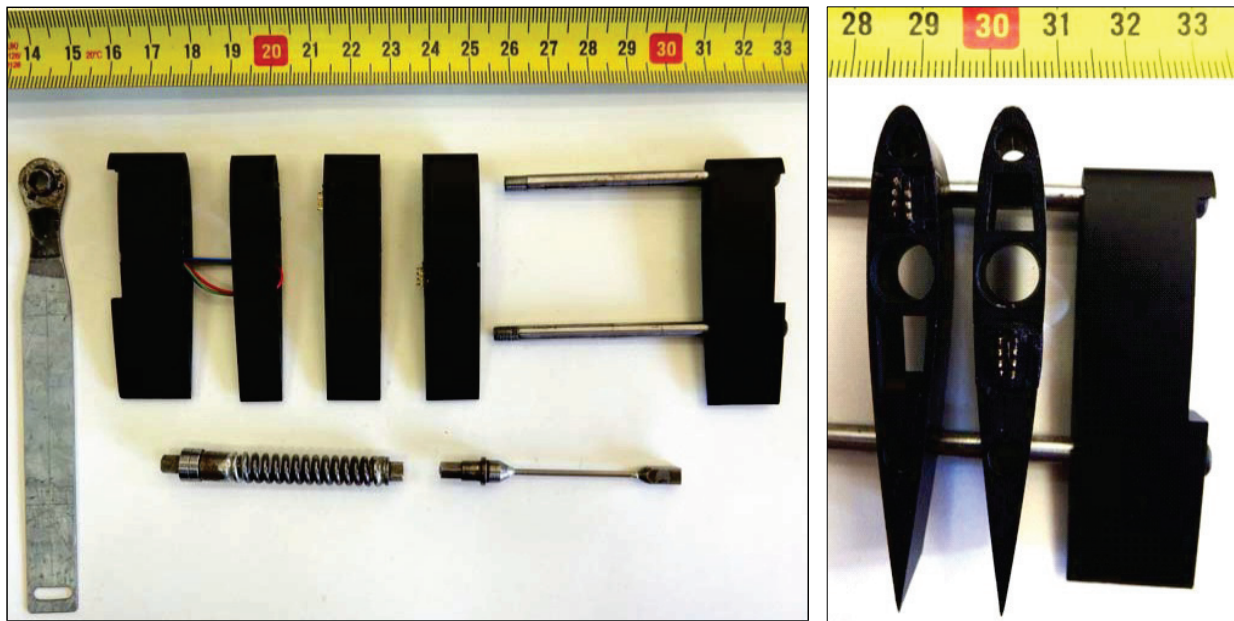
Fig. 1: Details and components of the measured profile: profile weight = 40.5/34 g (with the different axis); the axis of profile rotation is situated in 1/3 of the chord, measured from the leading edge; the instrument situated in the left part of the picture is used for zero position setting of the angle of attack.
