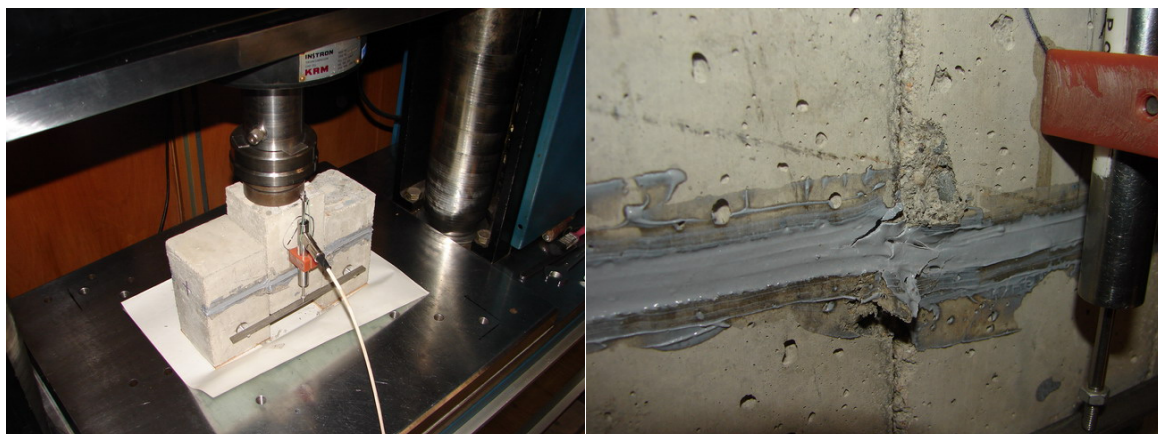
Fig. 1: View of the sample placed in a press and detail of the joint damaged by a shear force.
