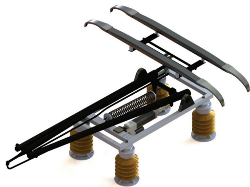
Fig. 1: The author's original concept model of pantograph
