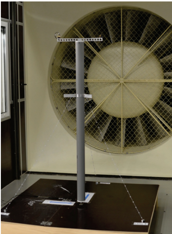
Fig. 2: The model of the guyed mast
