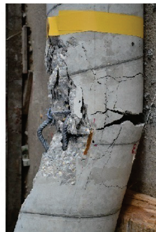
Fig. 3: Interaction diagram and failure of tested composite column
