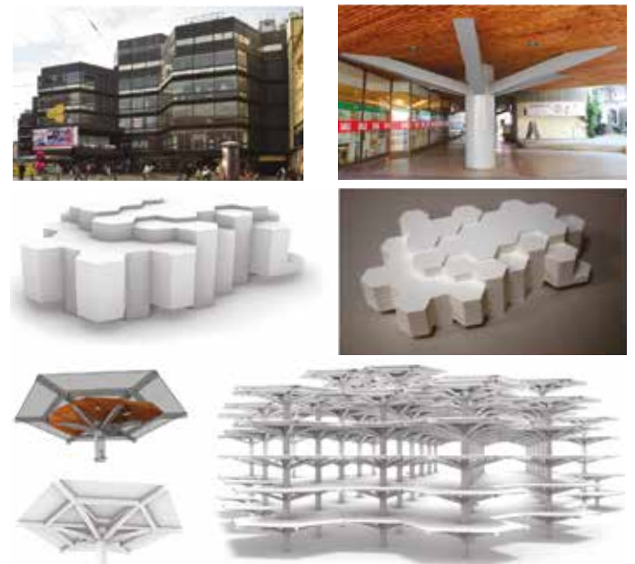
The digital documentation workflow: a volume model - from reality to 3D print (up), SCAN-to-BIM – pointcloud of the column from photogrammetry as a base for 3D modelling (bottom)
