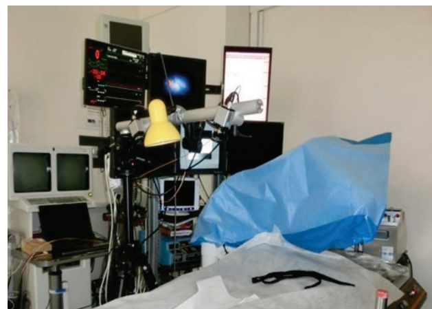
Fig. 3. Digital image stereo-correlation system with two cameras
