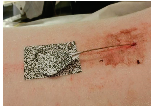
Fig. 2. Target with random pattern of black dots
