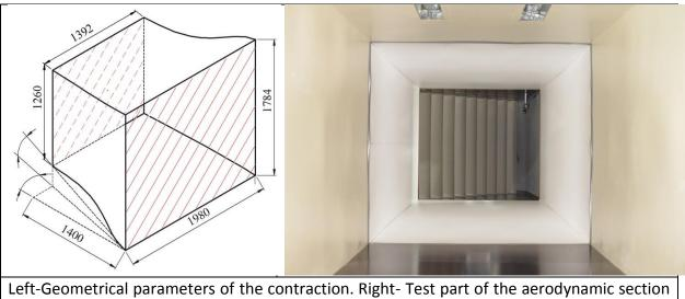
of the Climatic Wind Tunnel "Vincenc Strouhal" (downstream view)
