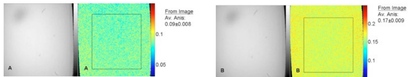
Figure 3. Calibration images are created by imaging FITC-loaded glycerol solutions of different concentrations. Higher glycerol concentration slows rotational diffusion rate to a greater extent, leading to higher anisotropy. A. Pseudo-color anisotropy image of 50% glycerol solution with mean isotropy of 0.09 \pm 0.008 (SD). B. Pseudo-color anisotropy image of 70% glycerol solution with mean isotropy of 0.17 \pm 0.009 (SD).
