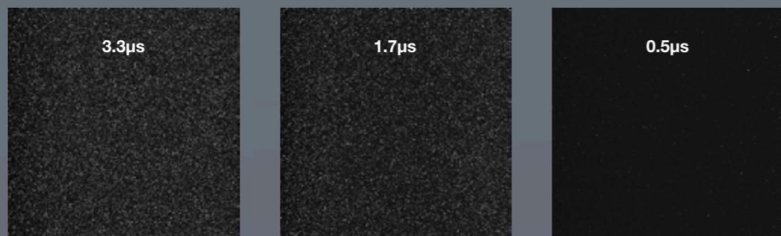
DARK IMAGES taken with the iXon3 897 at x1000 gain at different vertical shift speeds, 29 ms exposure time. Cooling temperature was -85°C to ensure minimal darkcurrent contribution.
