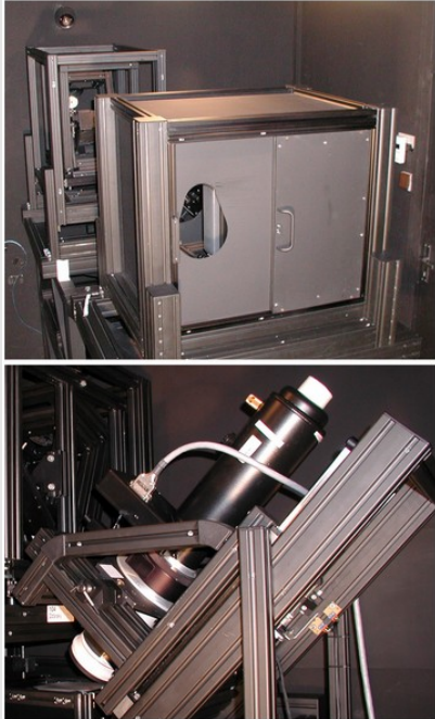
Fig. 2: Upper image - the mechanical parts holding the optical elements of the Ondřejov Echelle Spectrograph. Lower image - the detector with the dewar wessel. Credit: Miroslav Šlechta.
