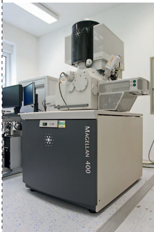
Extreme high-resolution SEM Magellan 400
