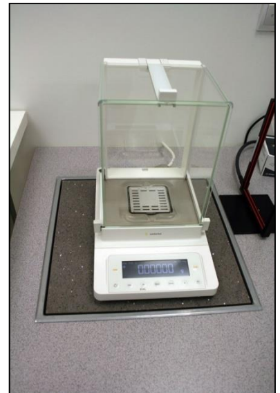
↑ Lab digital analytical balance scale is used for precise sample weighing.
