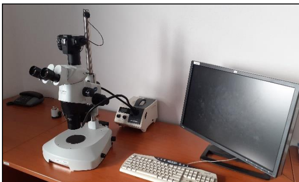
OLYMPUS SZX 16 Optical binocular microscope with the CANON digital photocamera and specialized QuickPHOTO Micro software and a Deep Focus module is used for the documentation of samples, various sample separations and imaging of objects.
