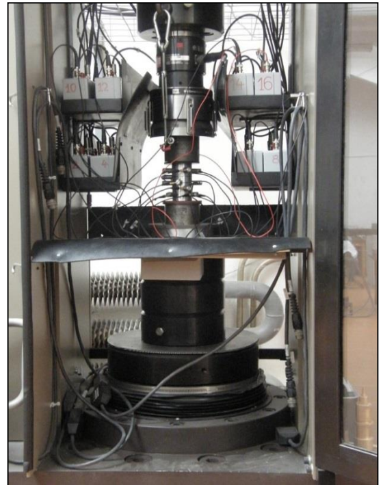
Uniaxial load frame MTS (max. force 4600 kN) is a computer-controlled servo-hydraulic loading system specifically adjusted for long-term testing. This system allows testing of rocks in regime of controlled force or controlled deformation. Together with triaxial cell, this equipment allows simulation of pressure-temperature conditions and permeability measurements.
