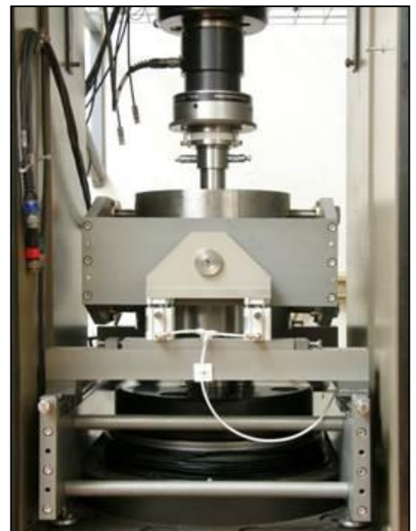
Uniaxial load frame MTS (max. force 4600 kN) is a computer-controlled servo-hydraulic loading system specifically adjusted for long-term testing. This system allows testing of rocks in regime of controlled force or controlled deformation. Together with triaxial cell, this equipment allows simulation of pressure-temperature conditions and permeability measurements.
