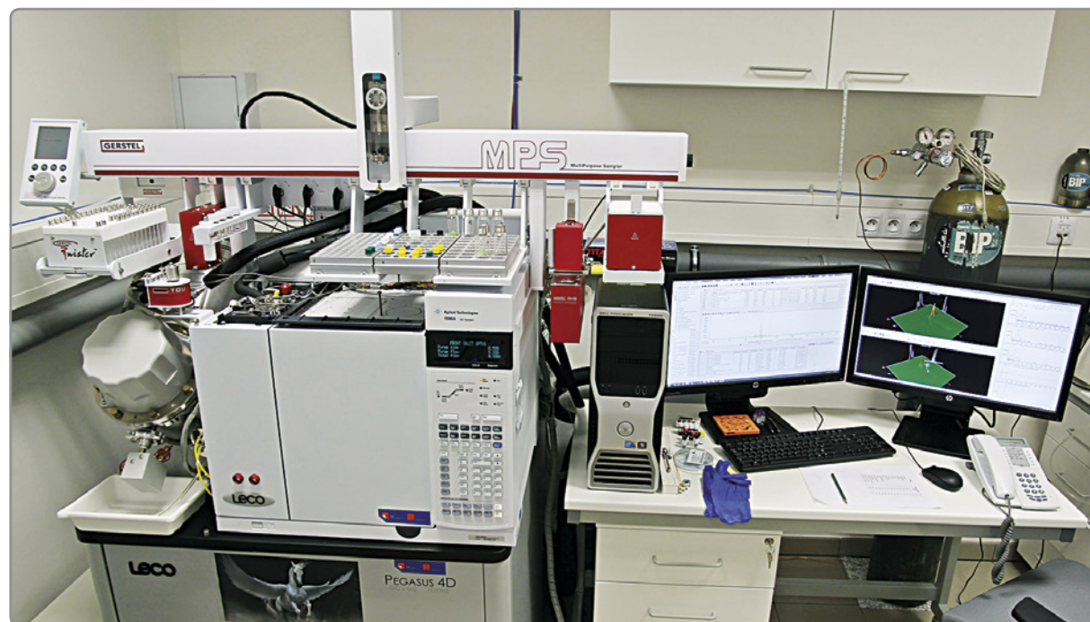
Figure 1: 2D gas chromatography coupled with mass detection will be performed on LECO Pegasus® 4D GCxGC-TOFMS system equipped with Cooled Injection System CIS 4 (GERSTEL), multipurpose sampler (GERSTEL) and Dynamic Headspace with Thermal Desorption Unit (GERSTEL). This equipment is used for precise analysis of predominantly hydrophobic and volatile compounds.
