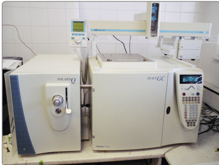
Figure 3: GC-MS system Polaris Q with Trace GC chromatograph and CTC combi PAL autosampler.
