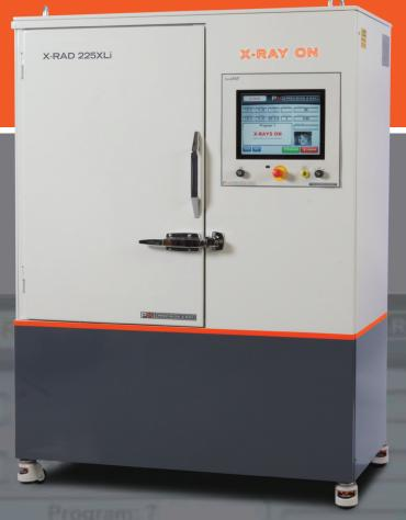
The X-RAD 225XLi has all the features of the 225XL but also includes the built-in OptiMAX M-IGRT imaging module, allowing high-resolution X-ray and optical multimodal imaging inside the cabinet.
