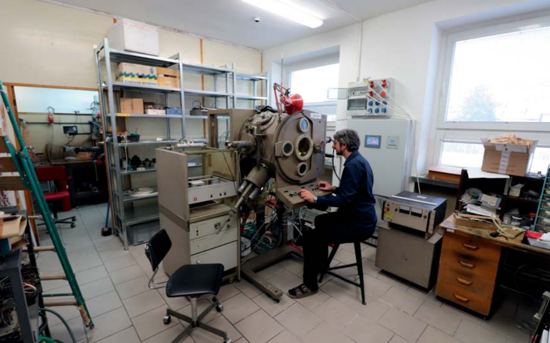
Electron beam welder
