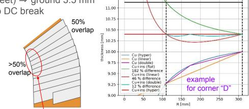
Different plate thickness at inner and outer radius  $\Rightarrow$  3D machining required. Is is possible to? (fiberglass tape allows compression  $\Rightarrow$ double roof shape sufficient)
