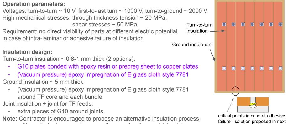
with equivalent or superior properties meeting the machining tolerances.
