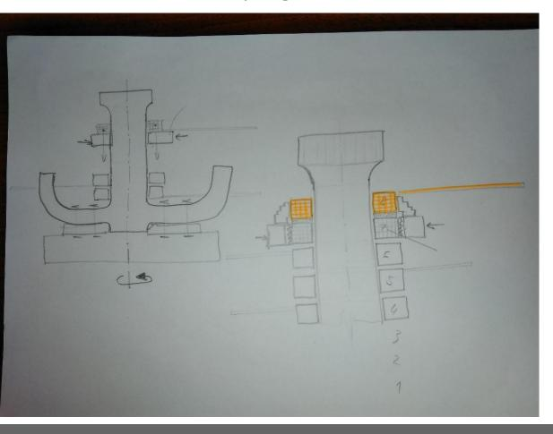
When winding, we need to protect the insulation of TF core. Ensure that the CS is wound on a protective tube (removable) Ensure that the CS winding / holding device does not destroy the TF core insulation during winding
