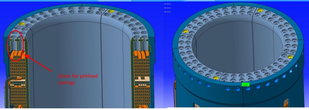
Can inner tie tube be used as vessel for VPI? Place for springs can not be glued same as coils to tie tube
