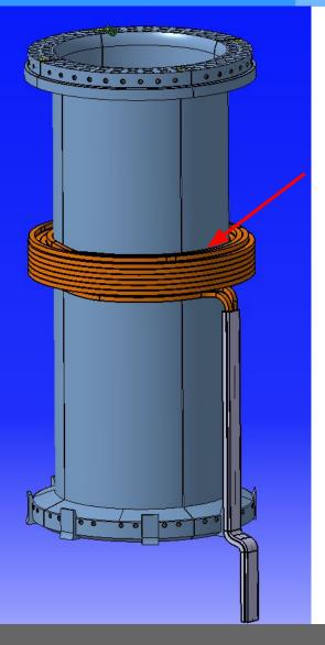
space between tie tube and coil's insulation is 1 mm This gap needs to stay free that CS coils can vertically move
