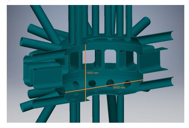
On picture (half section view), in green is shown space allocated for insulation.
