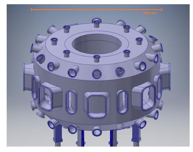
Overview of vacuum vessel. Space allocated for MLI is situated almost directly on the surface of the VV.
