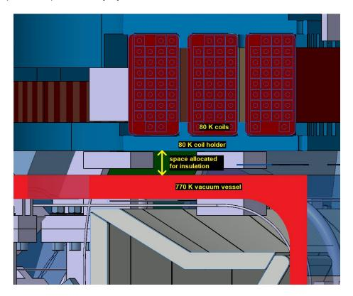
To make such construction possible, heat transfers between hot and cold parts must be carefully lowered. For initial phases available cryogenic cooling power will be about  $\sim$  10 kW, so it is important to keep heat load as low as possible.
