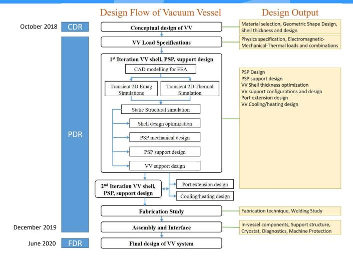
>The vacuum vessel is based on high normal and off-normal electromagnetic forces and thermal loads.
