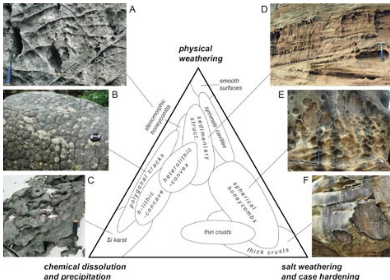
■ Fig. 25. A ternary diagram showing the estimated shares of physical weathering, chemical weathering and salt weathering for the individual morphofacies defined by the present research. Photos of some of the morphofacies defined: A – stenomorphonic honeycombs, Horní skály near Rynoltice, CR; B – polygonal cracks, Apremont-Bizons near Barbizon, France; C – siliceous karst, Larchant, France; D – accentuated sedimentary structures, Altschlossfels in Pfälzer Wald, Germany; E – large spherical honeycombs, Kamienie Brodzińskiego near Bochnia, Poland; F – thick rock crusts, Sokolka Hill near Branžež, CR (original).
