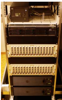
Fig. 1. The central file-server with 6.8 TB disk capacity (RAID 5).
