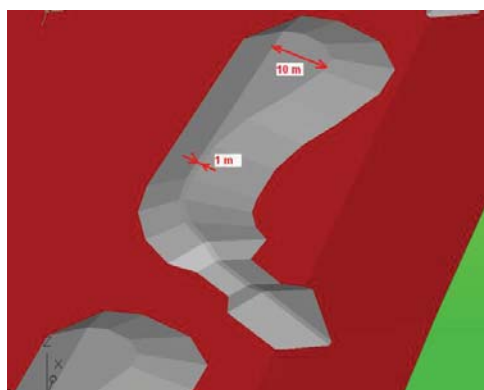
Fig. 3: Optimized spur dike.
