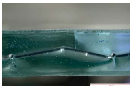
Fig.5: Notches caused by the cutting
