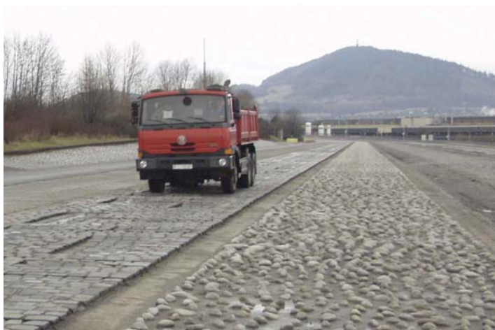
Figure 5. Test tracks on TATRA proving ground, vehicle is riding on the “belgická” test track, “buližník” track in front of the figure (Apetaur et al., 2009)
