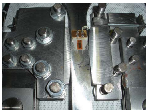
Fig. 4: Detail of the fretting pad installation in the experimental equipment – the original configuration without chamfers.
