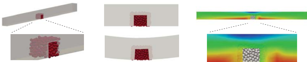
Fig. 9: Results of three point bending: initial state (a), undeformed and deformed final state (b) and normal stress (c)
