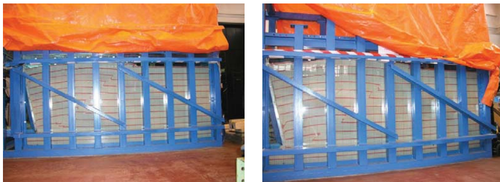
Fig. 3: View at right sides of the samples (granular masses of the same sand of size of 0.3 mm. a) Experiment E6/0,2 after toe movement of 212.3 mm (left). b) Experiment E5/0,2 after toe movement of 226.9 mm (right).
