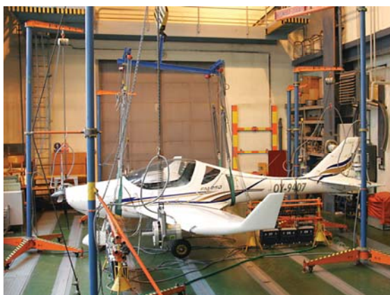
Fig. 2: GVT test arrangement (source: VZLU)
