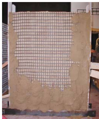
Fig. 2: Adobe brick wall with geo-nets (ABW_3)
