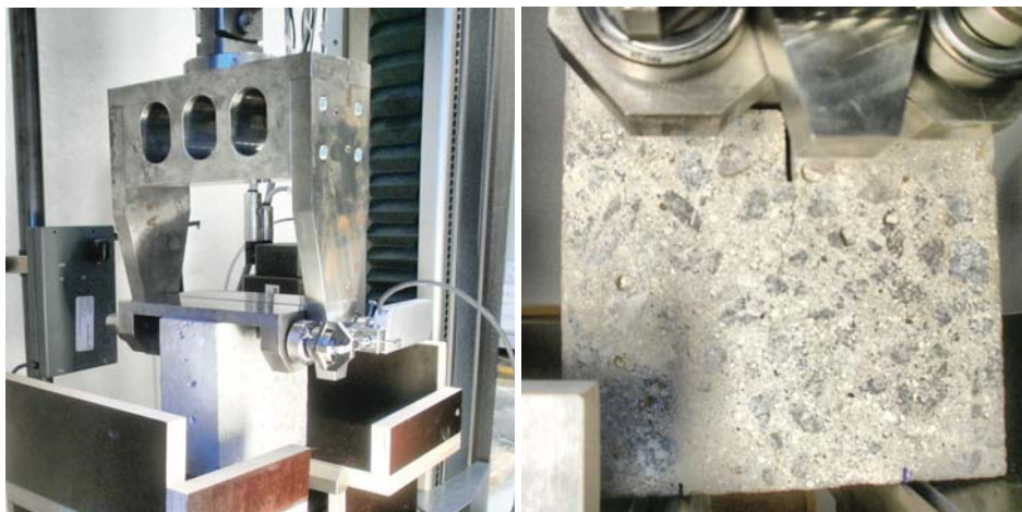
Fig. 2: Wedge-splitting test configuration and a detail of a cracked concrete specimen (photo by Táňa Holušová).
