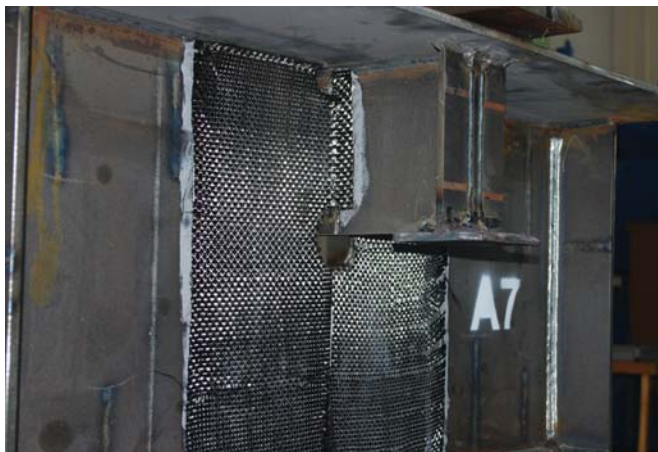
Fig. 10: The specimen A7 covered by the CFRC.
