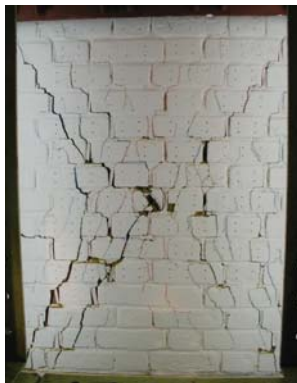
Fig. 7: Crack pattern at failure of the plain masonry control wall under a combination of vertical compression and cyclic shear. Fig. 8 - Envelope curves for unreinforced adobe wall (ABW_1).
