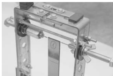
Fig. 1: Fastening of specimen to the acoustic device
