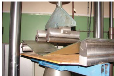
Fig. 2: Four point bending test on wire glass
