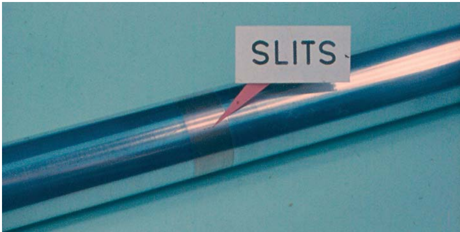
Fig. 13 (Right) Detailed photograph of the surface of the component M (see the next Fig. 14) and the flush fitting extensions. The diameter to length ratio of the complete assembly was satisfactory d/l = 0.1057 so that the local surface shear stress may be calculated from the known Blasius boundary layer solution for infinitely long round cylinder.
