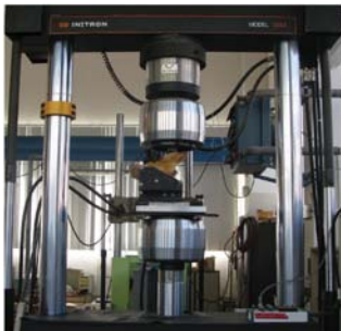
Fig. 6: The hip simulator
