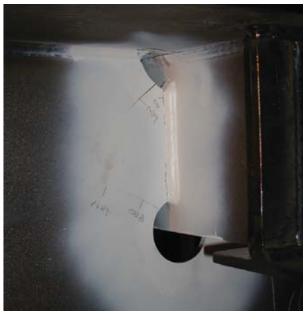
Fig. 4: Fatigue cracks on the specimen A2.
