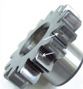
Fig. 1: Pitting damage of real gear.
