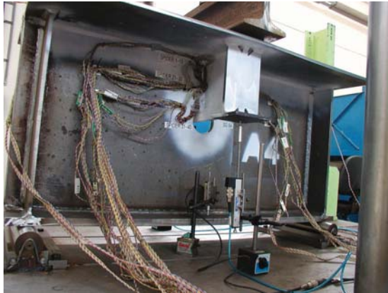
Fig. 7: The static tests on the specimen A 4 (arrangement for the hot spot method).
