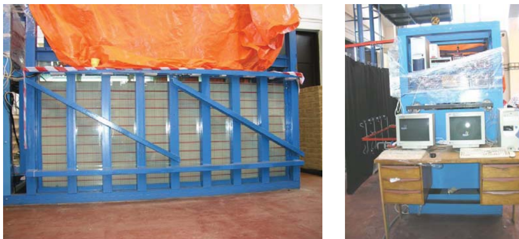
Fig. 1. Experimental equipment with transparent glass sides before experiment E6/0,2 with non-cohesive sandy sample into:
