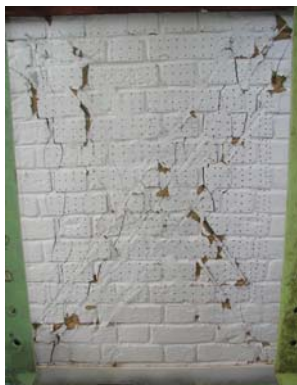
Fig. 9: Crack pattern at failure of the plain masonry control wall under a combination of vertical compression and cyclic shear.
