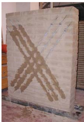
Fig. 3: Adobe brick wall with steel wire ropes (ABW_2)
