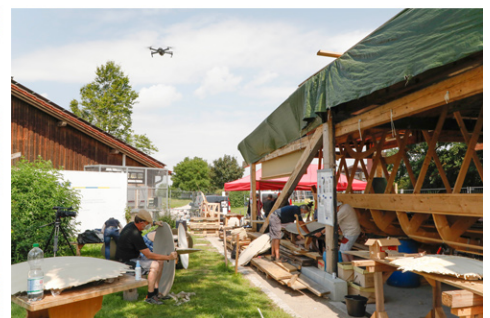
Photo middle below: To ensure that the wood has the right shape later, it must be extensively planed beforehand. It is a central process in Roman boat building (Photo by Giulia Iannicelli).
