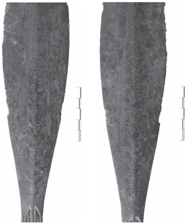
Fig. 3. Detail of the pattern-welded centre. Photo by G. Gattinger.
