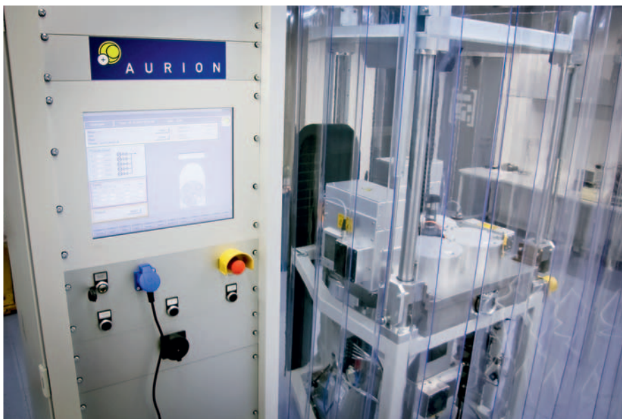
Computer controlled magnetron sputtering system Aurion
