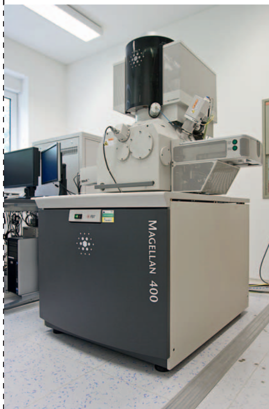
Extreme high-resolution SEM Magellan 400
