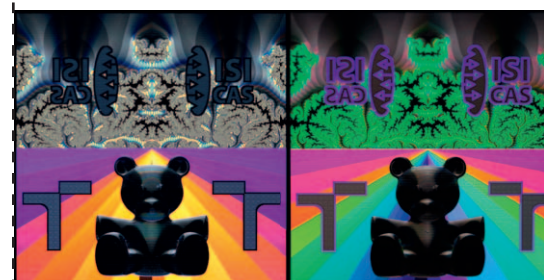
Example of a security hologram pattern in the layer of PMMA resist (left) and acrylic glass (right) specimens.
