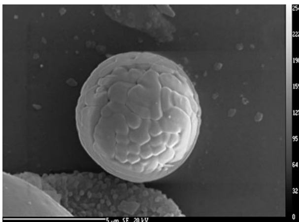
■ Fig. 42. Spherical magnetic object found in a sample of fly dust (Photo by Z. Korbelová).
