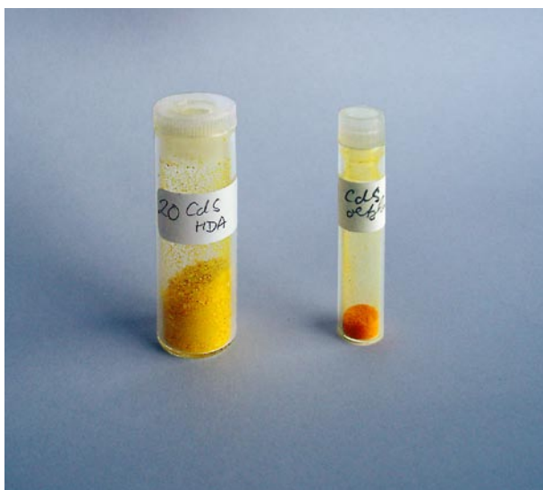
■ Fig. 16. Samples of CdS prepared in the course of the first year of the project solution (Photo by J. Rohovec).
