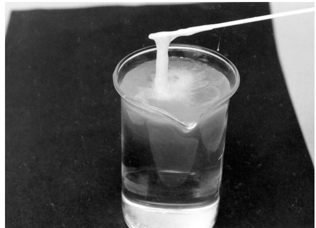
Fig. 1. Precipitation of PHEMA injected to water.
