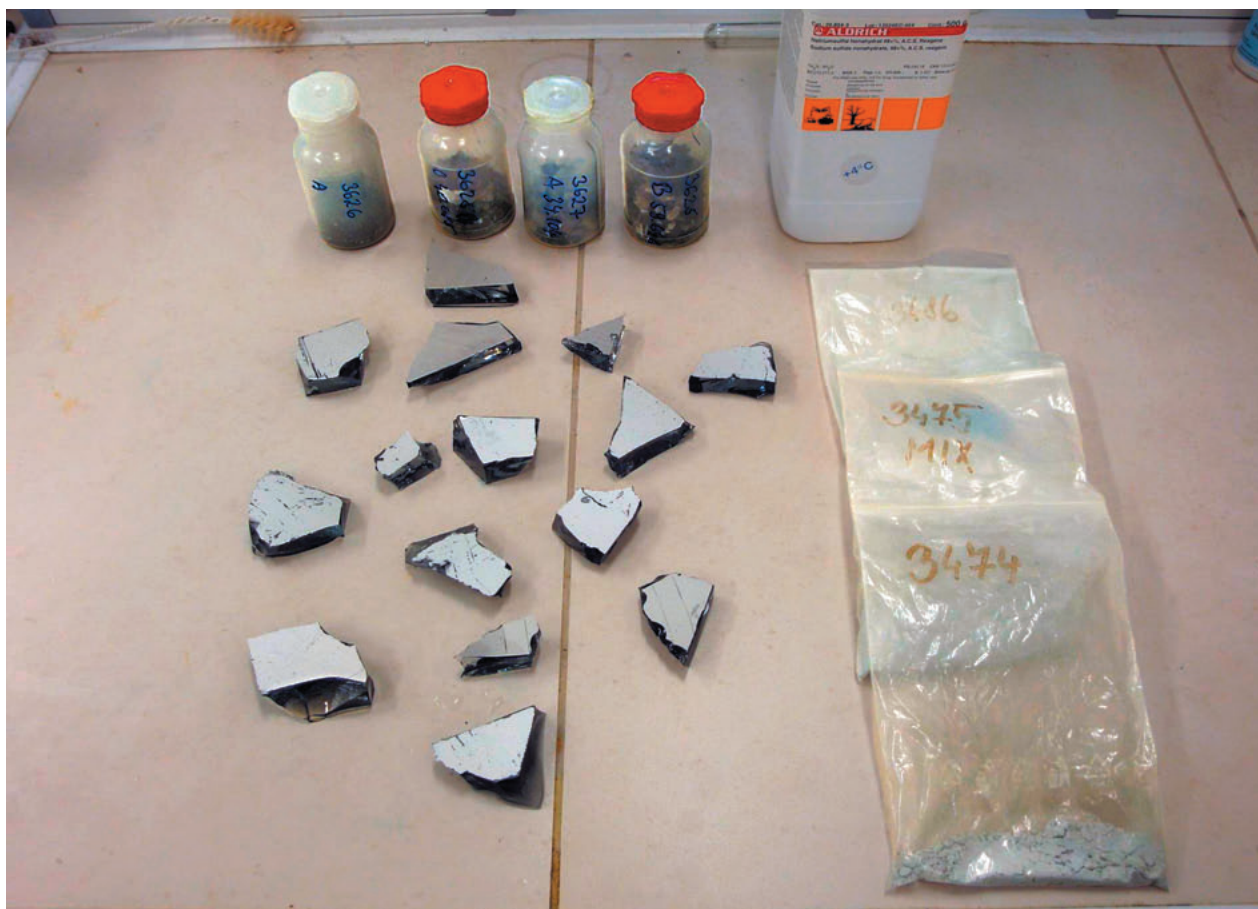
■ Fig. 14. Prepared large scale shards of CRT glass containing defined amount of the fluorescent coatings. Batch tests of scrap TV material in the 100ml bottles. Fine-grained crushed samples of cleaned TV screens in plastic bags. Photo by T. Navrátil.
