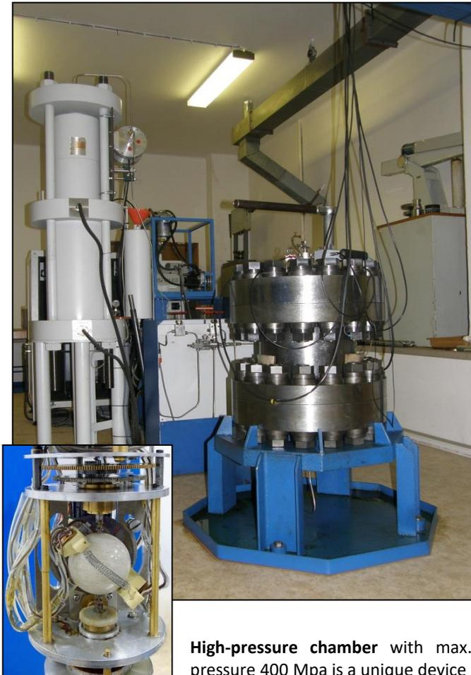
**High-pressure chamber** with max. pressure 400 Mpa is a unique device
