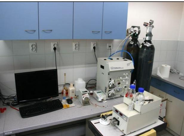
The **PS-Analyser** instrument is designed for mercury analyses in liquid samples and for speciation studies with HPLC separation.
