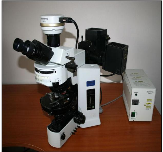
**OLYMPUS BX50** Optical polarizing microscope with the **DP 70** digital camera and specialized **QuickPHOTO** software and a **Deep Focus module** is used for a detailed study of thin (for transmitted light) and polished (for reflected light) sections. Software enables documentation, image preparation and image analysis. The microscope is equipped also with a fluorescent source of different wavelengths.
