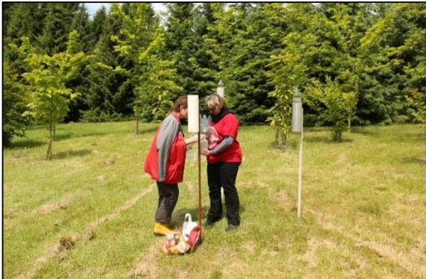
Collection of an environmental sample: **Passive collector** for collection of rain water.
