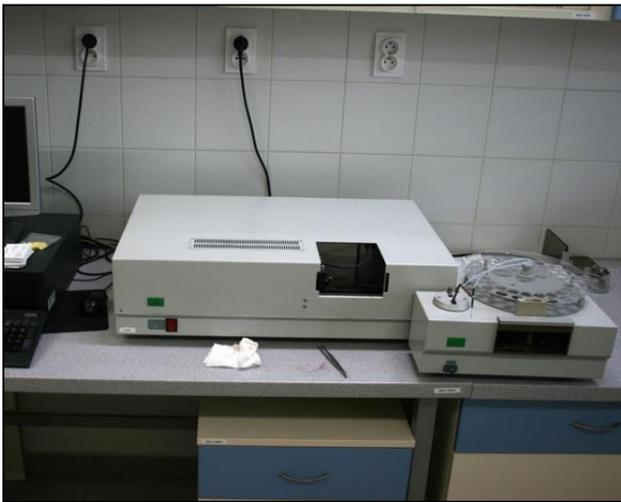
The **AMA 254 advanced mercury analyser** is our basic instrument used for analyses of mercury contents in solid samples without need of prior sample preparation. At present, we are running two of these units. First one is used for Hg analyses in soil horizons, various biomass and general samples, while the second is used solely for readout of Hg content in wood of tree rings in projects dealing with tree ring geochemical archives.
