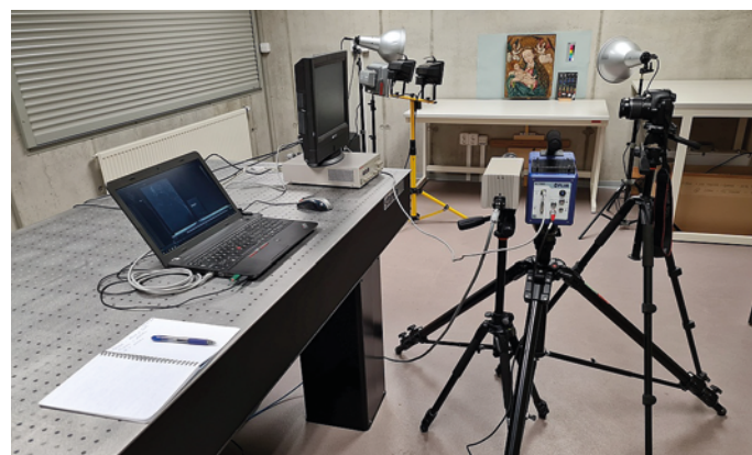
Lamp set with thermal imager and IR camera for image documentation at the Optical Methods Laboratory in Telč. Photo: J. Valach.
