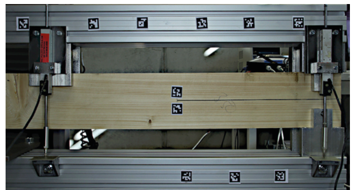
Experimental set up for mixed mode is labeled by aruco markers for stiffness assessment by optical methods.
