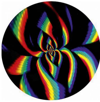
Diffractive Optical Variable Image Device (DOVID) using phyllotaxy arrangement. Real photo (left), light microscope image (right).
