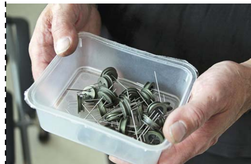
Electrical vacuum feedthroughs
