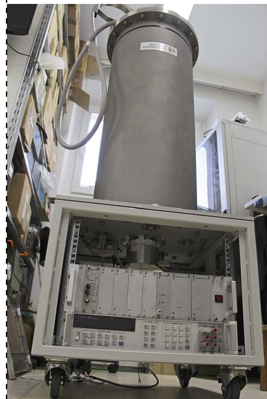
High voltage reference divider for voltages up to 120 kV
