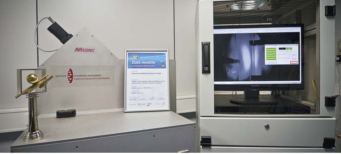
Contactless laser interferometer system for gauge block calibration awarded Gold medal of 54th International Engineering Fair in Brno
