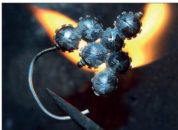
Obr. 6/235: Granulace se pájela vždy po jedné straně. Fig. 6/235: Soldering of granulation is always performed first on one side, than the other.
