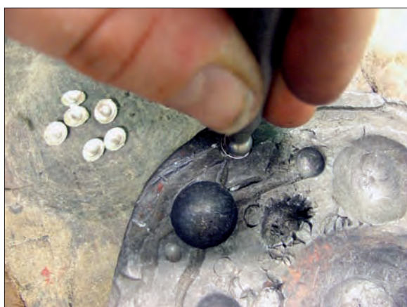
Obr. 6/127: Tepání puklic v jamkovnici. Fig. 6/127: Embossing the hemispheres on the lead block.
