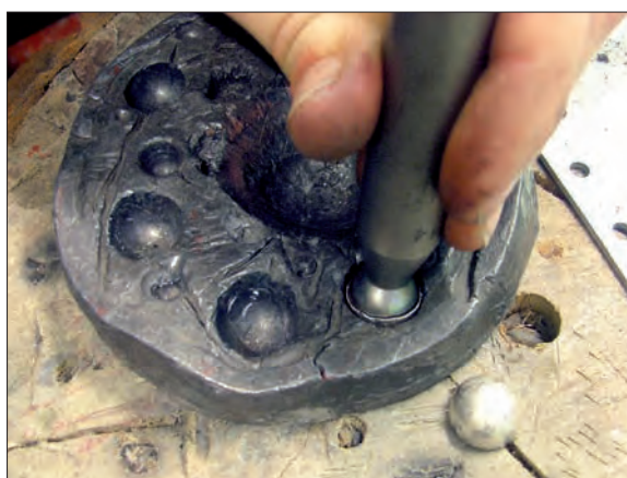
Obr. 6/126: Tepání čakanem v jamkovnici. Fig. 6/126: Embossing the hemisphere in the lead block with a dapping punch.
