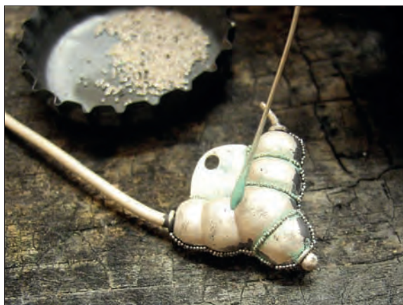
Obr. 6/203: Nanesení granulí do prohlubní reliéfu s difuzní pájkou. Fig. 6/203: Setting of granules between the pseudo-globes by application powder of malachite mixed with gum tragacanth.
