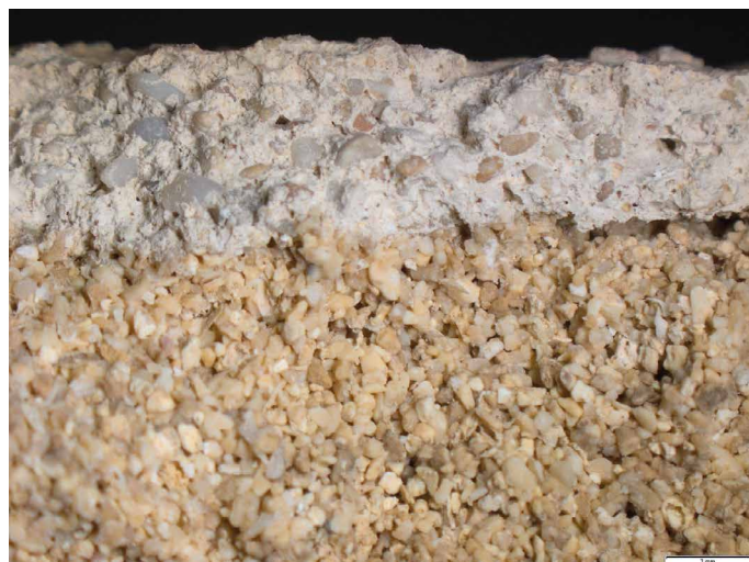
Sample YSC 18, a gypsum mortar laid on top of a sandstone. The sample was collected from Yeronisos Island and is supposed to be from the Hellenistic period. Photo: P. Pizzo
