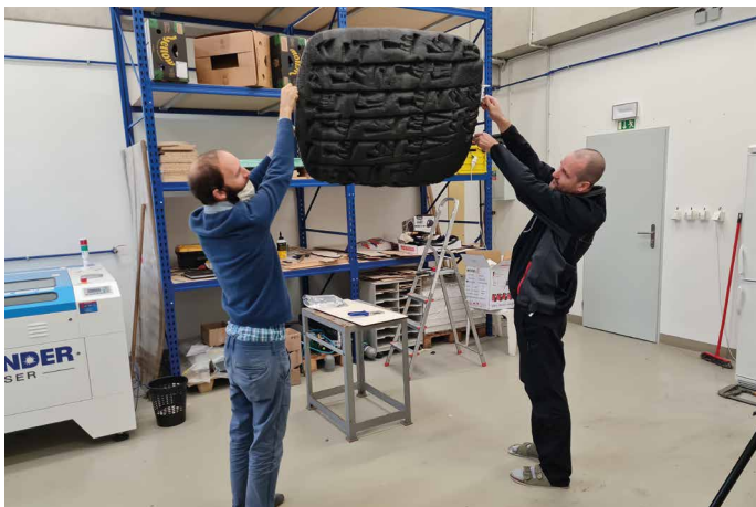
Preparation of the exhibition: 50-times enlarged cuneiform tablet made of glued-together layers of PU foam laser cut according to a digital 3D model.
