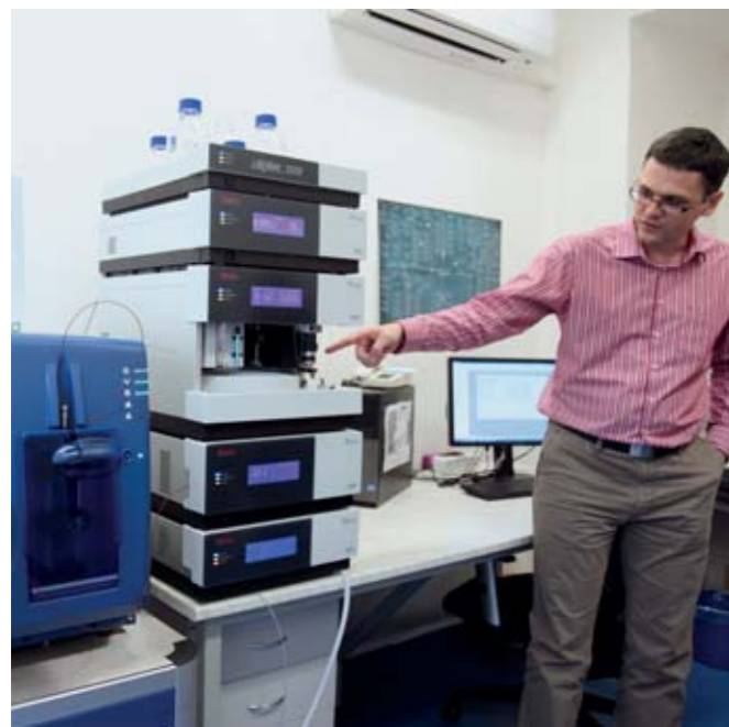
The Institute of Physiology of the ASCR on 16 October 2012 introduced its new peak mass spectrometer QTRAP 5500. The new magnifying device, which is one of the hybrid mass spectrometers, systems merging a triple quadrupole and a linear ion trap, allow a detailed analysis of the activity of consumed foods or medicines on the tissue and cellular metabolic systems.
