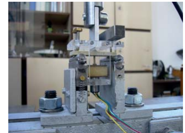
Testing of the flexural strength of the consolidated stone plate. Testing of mechanical characteristics of historic building materials before and after the treating with the liquid strengthening agents is a basic technique allowing the evaluation of the consolidation effect of these agents, which are often impregnated into weathered building facades for lifetime prolongation. (Institute of Theoretical and Applied Mechanics)
