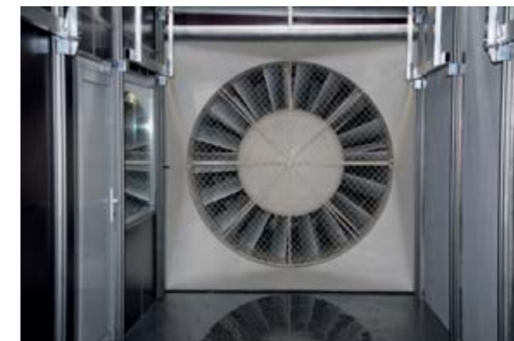
The climate tunnel in the Centre of Excellence Telč. In the picture, the climate chamber with a 200kW ventilator. The chamber is prepared for attaching the samples into the openings in the flooring. The moveable ceiling allows operational manipulation with the water nozzles or radiant lamps.
