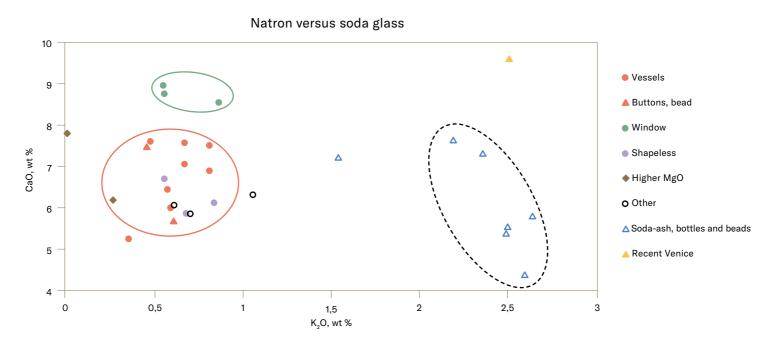
Fig. 254 Comparison of the chemical composition of the natron glass and soda-plant ash glass. Venetian glass lies outside of both the sets.
