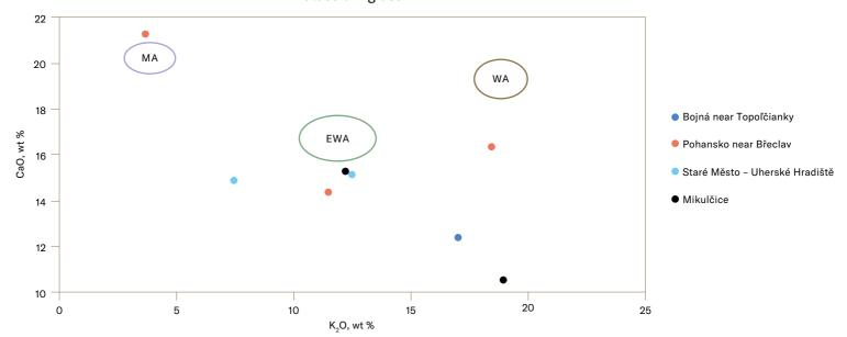
Fig. 255 The  ${\rm CaO/K_2O}$  ratio in potassium-calcium glass. The large variability in the composition is related to the ash used and also with the ratio of raw materials in the glass batch (i.e. raw materials prepared for melting). Potassium glass comes from the Northern Alps – Western Europe.
