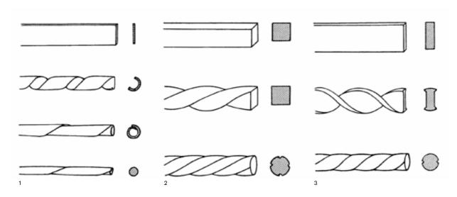
Fig. 102 Three ways to produce round wire.
