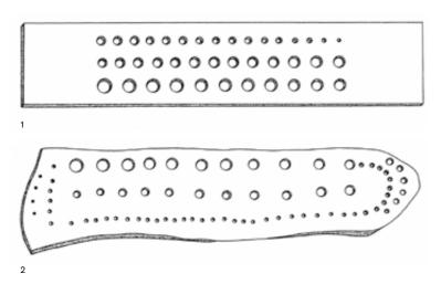
Fig. 101 Draw-plates for the production of round wire.
