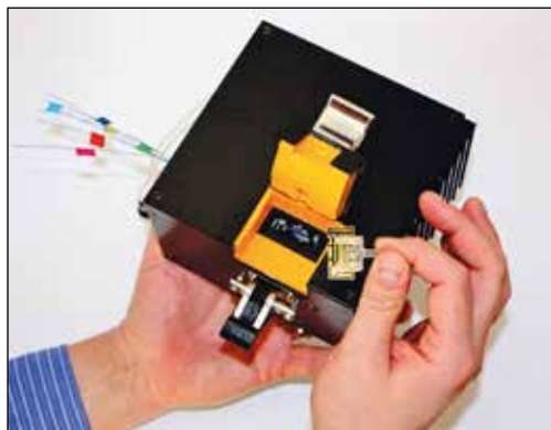
Fig. 3 Photograph of a prototype of the compact SPR biosensor based on SPRCD element incorporated in a plastic cartridge
