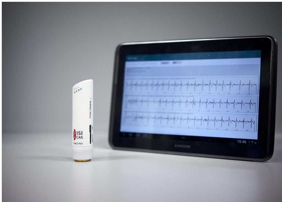
A hand-held device for instant screening of the heart activity (HACT-FV3) implements machine learning embedded on the FPGA chip
