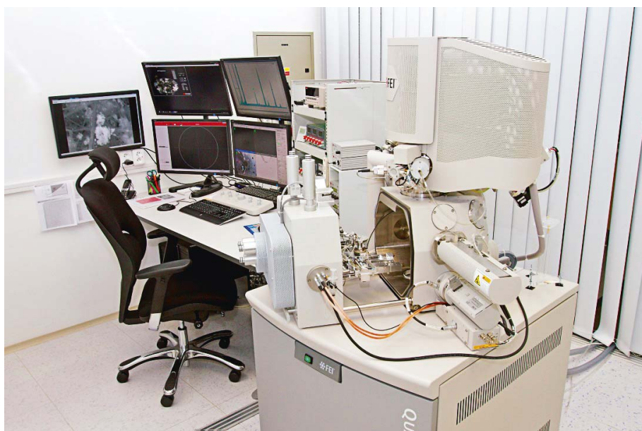
Laboratory of environmental electron microscopy with high resolution ESEM QUANTA 650 FEG (left) equipped with micromanipulators (right)
