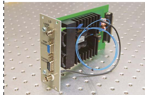
Highly coherent semiconductor laser for the telecommunication applications
