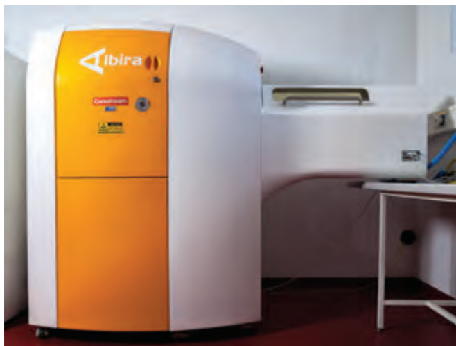
The \mu CT/PET scanner for small animals (Albira, Bruker). This instrument enables the preclinical morphological and functional imaging of small laboratory animals such as mice or rats with high spatial resolution.
