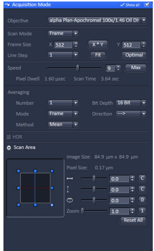
Fig. 135 Acquisition Mode - Frame with LSM tab selected in the Imaging Setup tool
