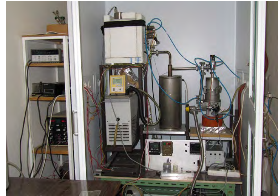
Fig. 6: Prototype of a STAT 7 apparatus for the exact measurement of vapor pressures of metal-organic precursors developed in the frame of cooperation between the Institute and the Institute of Chemical Technology, Prague. Similar version of this model was also installed in 2011 in the NIST (formerly Bureau of Standards, USA) as an étalon apparatus.
