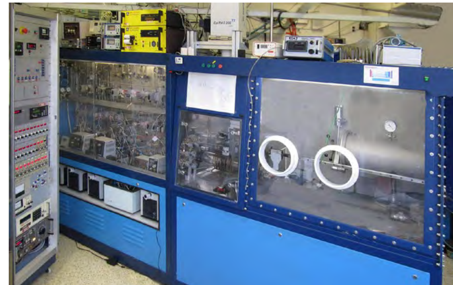
Fig. 1: The first commercial MOVPE apparatus AIXTRON 200 in the Czech Republic was taken over in 1994 from AEG–Ulm, Germany and installed in the Department of Semiconductors.
