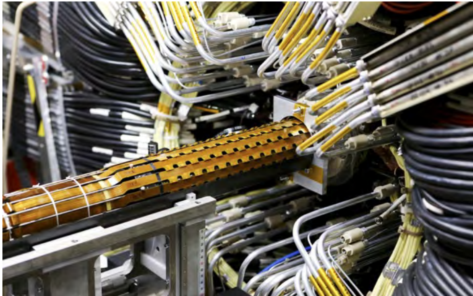
Fig. 2: Insertable B-Layer – new layer of pixel detectors was added to the ATLAS inner tracker detector during the last LHC shutdown. Institute of Physics contributed to the development, construction and installation of this device.
