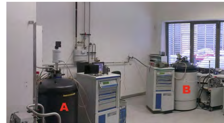
Fig. 2: Physical Properties Measurement Systems equipped with 9 T (A) and 14 T (B) superconducting coils, Joint Laboratory for Magnetic Studies
