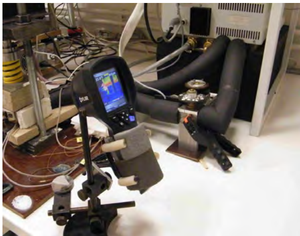
Fig. 3: Automated characterization equipment for testing of thermoelectric modules and materials.
