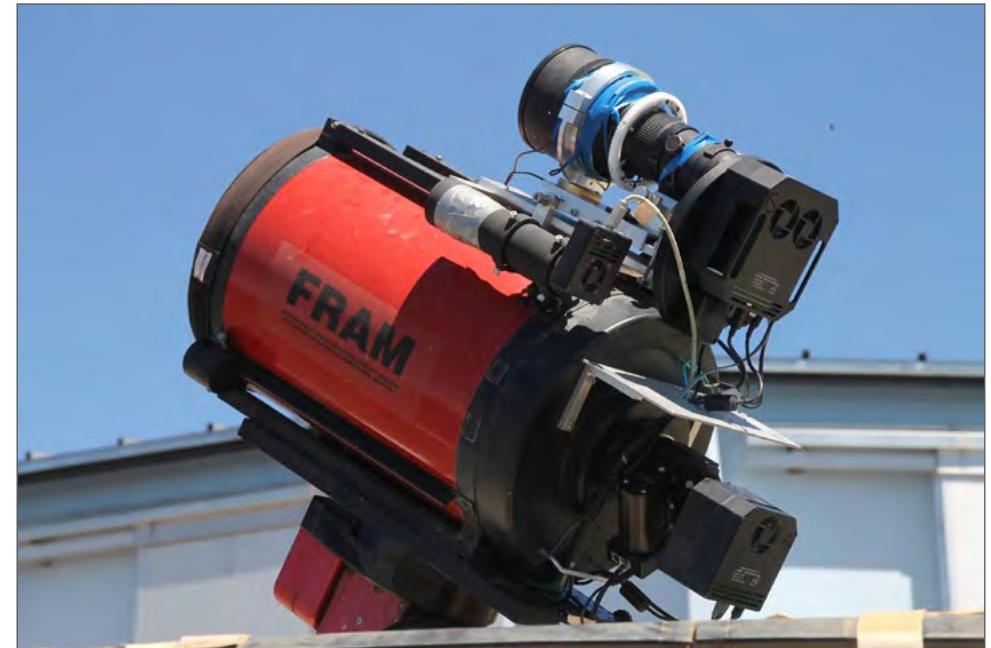
Fig. 2: FRAM (F/Photometric Robotic Atmospheric Monitor), seen here next to the Los Leones fluorescence telescope building is a robotic astronomical telescope capable of automatic monitoring of atmospheric conditions in various parts of the sky, including fast follow-up observations along the trajectory of a recently observed air shower. The telescope, its supporting infrastructure and the operating software have been developed by the Institute.
