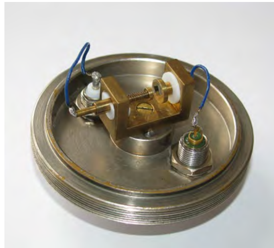
Fig. 7: Sample holder for realization of the point contact to high resistance materials enabling one to measure parameters otherwise inaccessible by magnetotransport methods.
