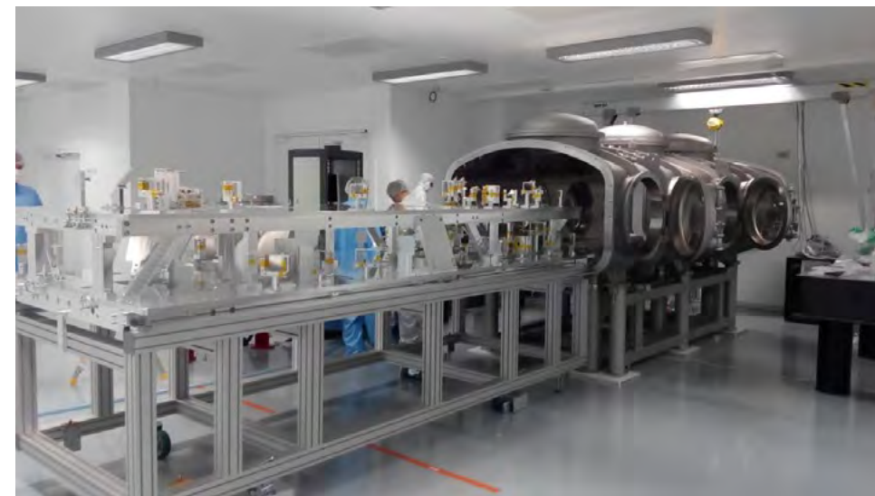
Fig. 1: Assembling the ps vacuum compressor for the L1 laser of ELI-Beamlines, designed by the Dept 91 research and technical team, in cooperation with engineering support by Dept. 93.
