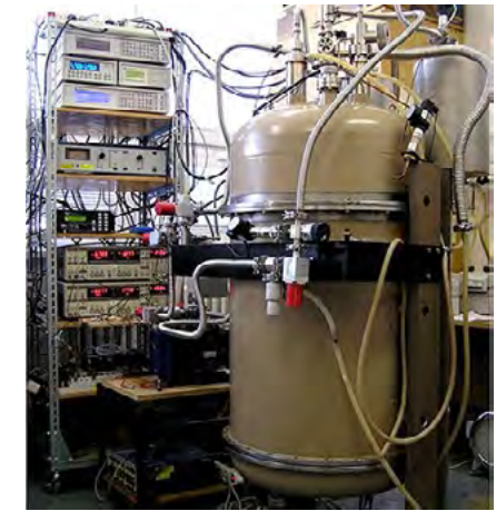
Fig. 1: Apparatus for generation of quantum turbulence, Joint Laboratory of Low Temperatures
