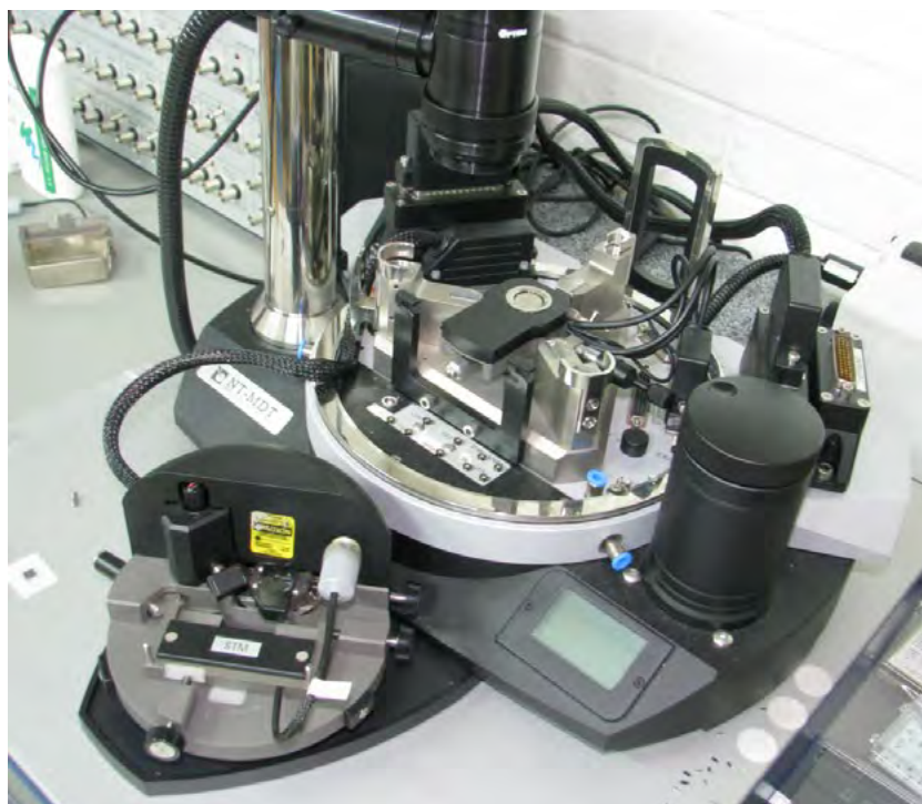
Fig. 7: Atomic force microscope setup for measurements of proteins and nanoparticles.
