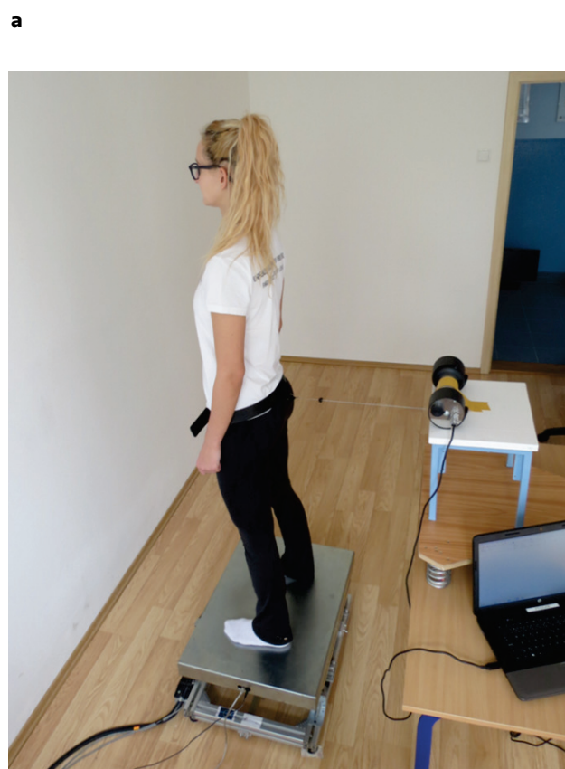
Fig. 1. (a) FITRO Dyne Premium and FITRO Dynamic Posturography system and an example of on-line display (b – above) of peak velocity and range of trunk movement and (b – below) velocity of platform translation with corresponding acceleration.
