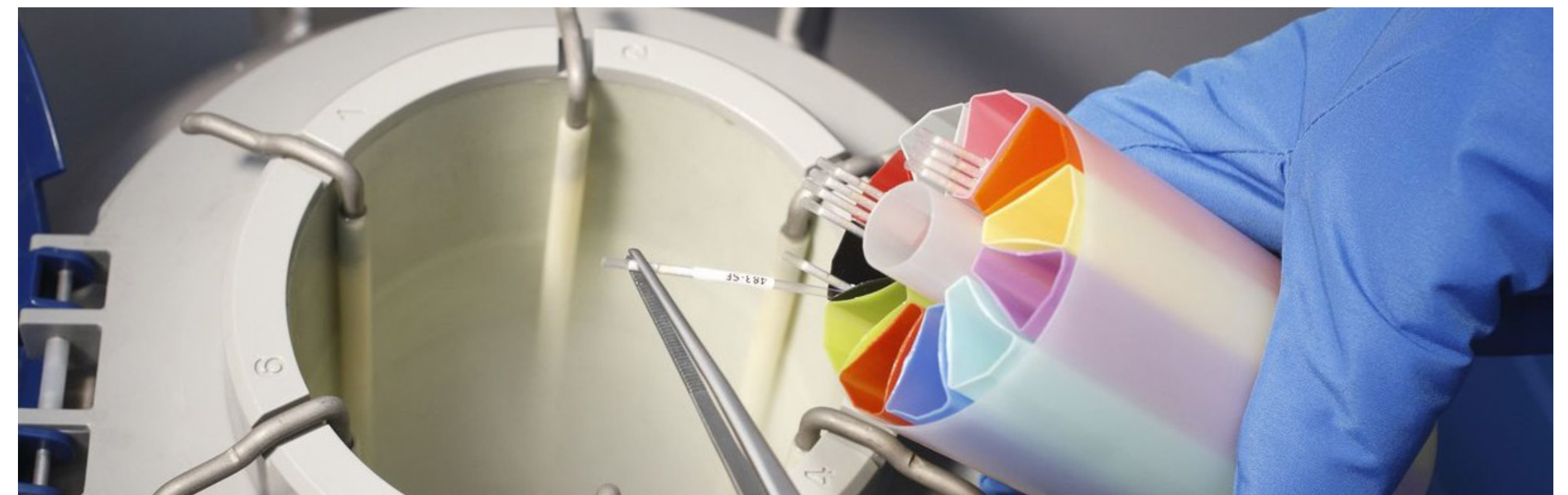
Mobile dewar LS750 Taylor-Wharton used for mouse sperm freezing and goblet system for long storage in LN 2 .
