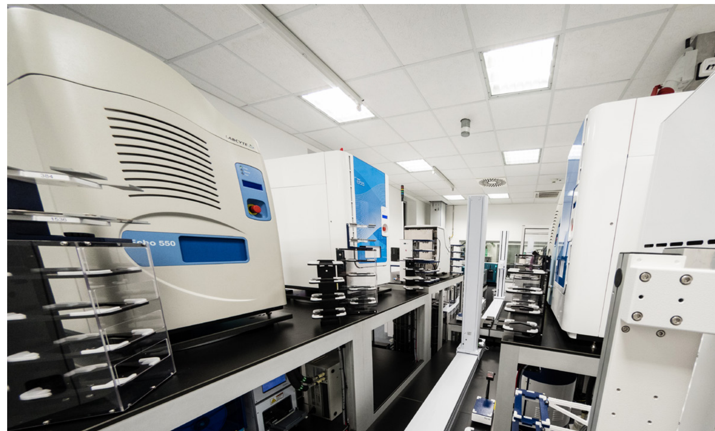
The acoustic compound transfer unit is part of the High-throughput screening system.
